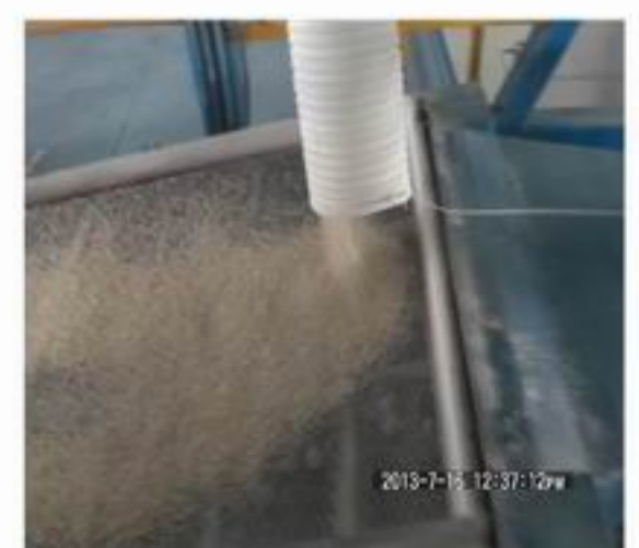
Stage 1 Material distribute at inlet
